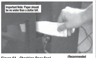
Figure 51 - Checking Door Seal
